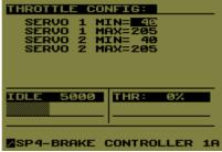
**MIN THROTTLE:** starting position for the servo when THR=0%. In steps of 1/255. You have to ensure the throttle is completely closed at this position (consider engine's idle adjust). In this option the LEFT knob is use to change the value.
