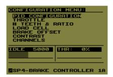
PID configuration: These values are used to control the engine RPM at Steady RPM and RPM Ramp modes. KP-proportional, TI-Integral, TDderivative. They can be changed with the left knob. Its performing is explained later.
