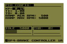
Ramp min, and max values are also in this window, these values are used in the ramp mode as limits to the ramp auto-increment. When the engine decreases its speed (because throttle is closed) the system detects this condition and decreases automatically the target rpm, this value is limited by the "ramp min" value. When the engine is accelerating, the target value is increased automatically at the ramp rate until the "ramp max" value is reached.
